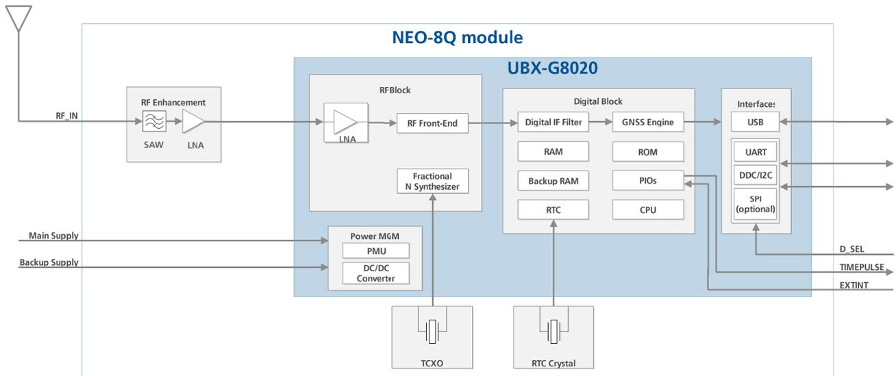
Figure 1: NEO-8Q block diagram
