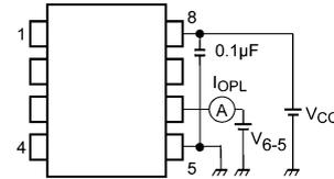
**Fig. 13.1.2 I<sub>OPL</sub> Test Circuit**
