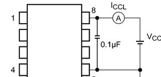
**Fig. 13.1.6 I<sub>CCL</sub> Test Circuit**
