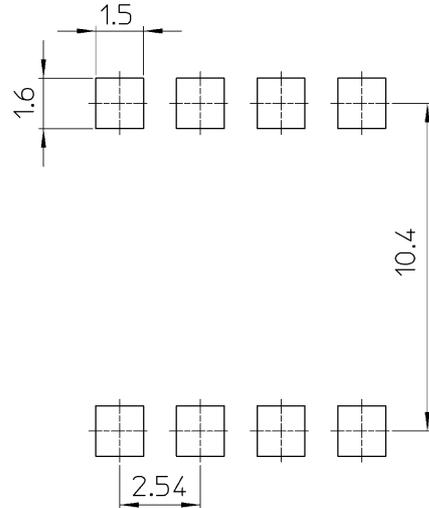
**Fig. 15.2 Lead forming and taping option (LF4), (TP4)**
