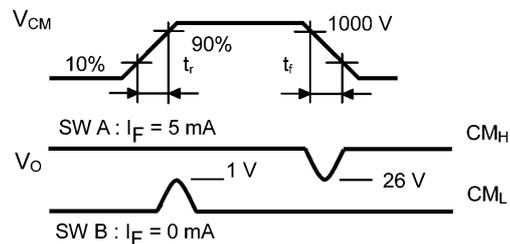
$$CM_L = \frac{800(V)}{t_r(\mu s)} \quad CM_H = -\frac{800(V)}{t_f(\mu s)}$$
