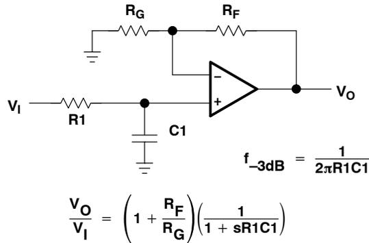
**Figure 50. Single-Pole Low-Pass Filter**
