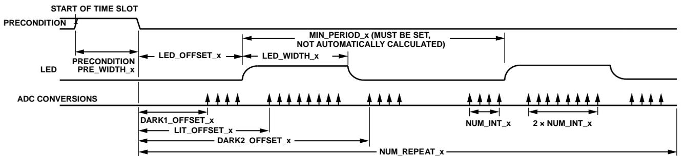
Figure 47. Two-Region Digital Integration Mode Timing Diagram
