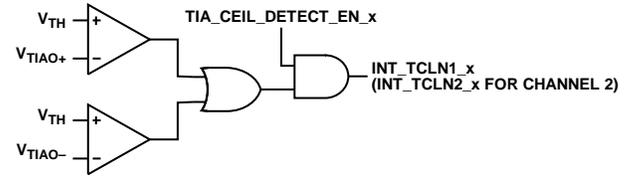
Figure 50. Schematic of TIA Ceiling Detection Circuit
