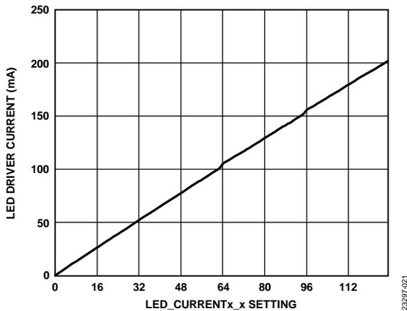
Figure 20. LED Driver Current vs. LED\_CURRENTx\_x Setting
