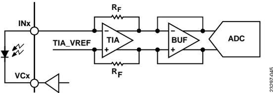
Figure 45. Signal Path for Digital Integration Mode
