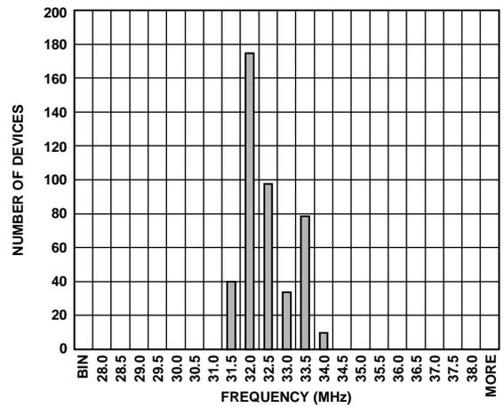
Figure 15. 32 MHz Clock Frequency Distribution, Untrimmed
