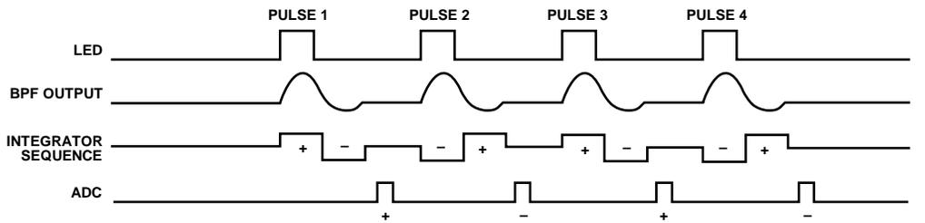
Figure 36. Diagram of Integrator Chopping Sequence
