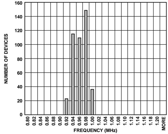
Figure 14. 1 MHz Clock Frequency Distribution, Untrimmed
