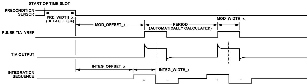
Figure 43. Timing Diagram for Self Capacitance-Based Proximity Measurement
