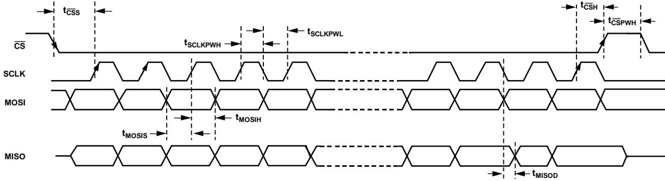
Figure 3. SPI Timing Diagram for the ADPD4101
