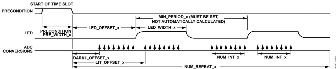
Figure 46. One-Region Digital Integration Mode Timing Diagram
