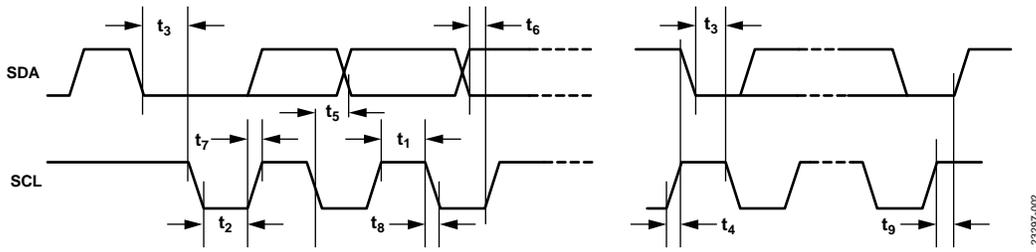
Figure 2. I<sup>2</sup>C Timing Diagram for the ADPD4101
