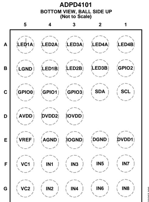
Figure 5. ADPD4101 Pin Configuration
