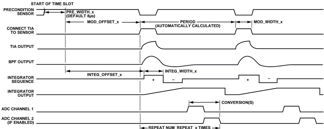
Figure 40. Timing Diagram for Pulse Connect Modulation
