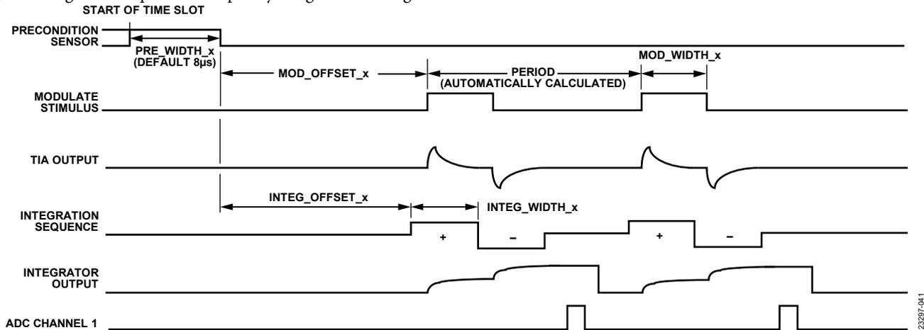
Figure 41. Timing Diagram for Modulate Stimulus Operation
