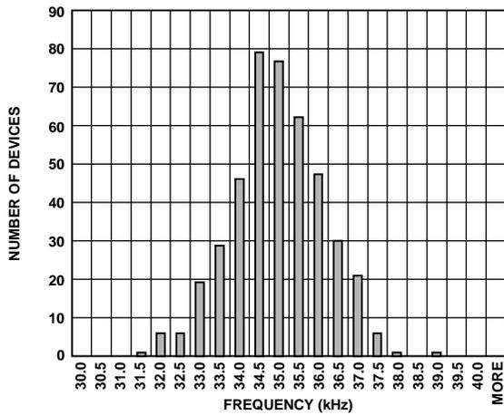
Figure 13. 32 kHz Clock Frequency Distribution, Untrimmed
