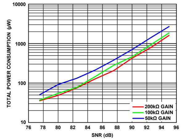
Figure 11. Total Power Consumption vs SNR in Continuous Connect Mode Including LED Power,  $C_{PD} = 70$  pF, Integrator Input Resistor = 400 kΩ, ODR = 25 Hz, CTR = 150 nA/mA, LED Supply Voltage = 4 V, 90% of Full Scale
