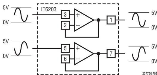
**Figure 8. LT6203 Buffering a Fully Differential Signal Source**
