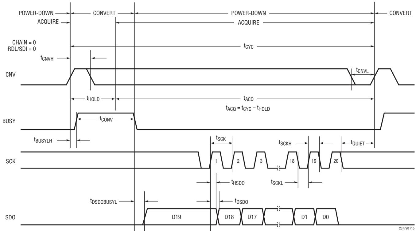
Figure 15. Using a Single LTC2377-20 in Normal Mode
