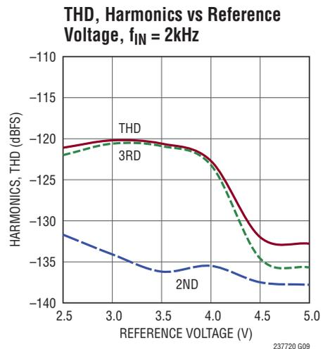
**TYPICAL PERFORMANCE CHARACTERISTICS**  $T_A = 25^\circ\text{C}$ ,  $V_{DD} = 2.5\text{V}$ ,  $0V_{DD} = 2.5\text{V}$ ,  $V_{CM} = 2.5\text{V}$ ,  $REF = 5\text{V}$ ,  $f_{SAMPL} = 500\text{ksps}$ , unless otherwise noted.
