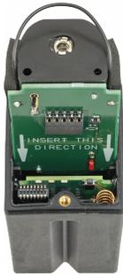
Figure 5: Q45 battery board for c-cell batteries
