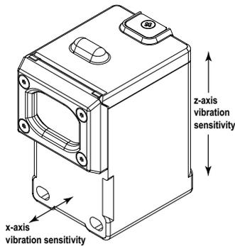
The vibration sensors have an x- and z-axis indication on the face of the sensor.
