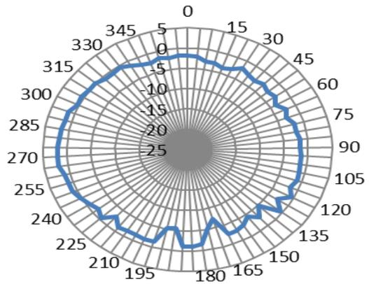
**FIGURE 4.5.3 2D RADIATION PATTERN OF ANTENNA AT 5.5GHZ IN FREE SPACE FOR CONFIGURE 2**
