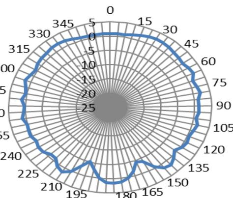
**FIGURE 4.5.1 2D RADIATION PATTERN OF ANTENNA AT 2.4GHZ IN FREE SPACE FOR CONFIGURE 1**
