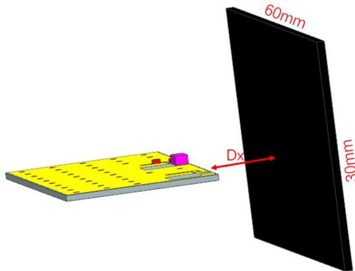
**FIGURE 7.2 FOUR LOCATIONS WITH VERTICAL PLANE GROUND (USING CONFIG1 FOR ILLUSTRATION)**
