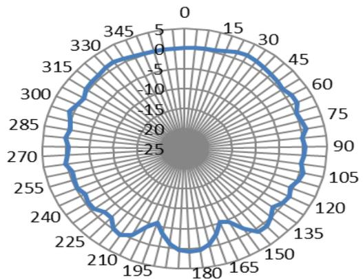
**FIGURE 4.5.2 2D RADIATION PATTERN OF ANTENNA AT 2.4GHZ IN FREE SPACE FOR CONFIGURE 2**
