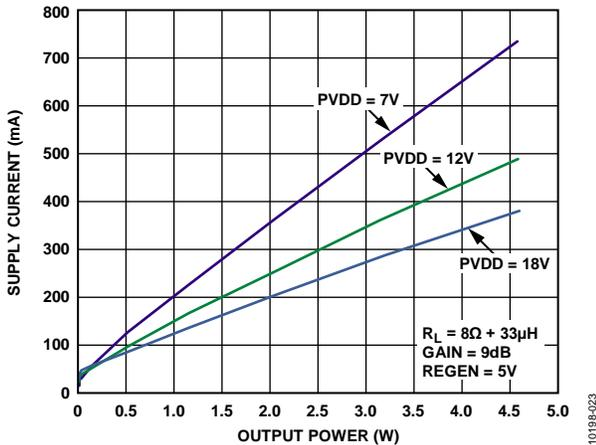
Figure 23. Supply Current vs. Output Power into 8Ω;
