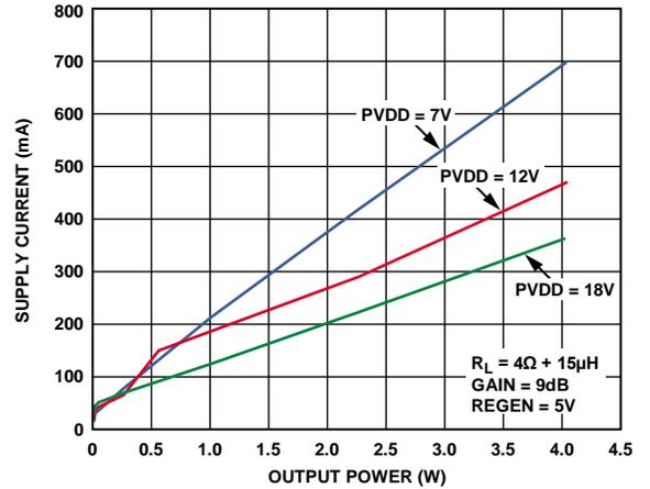
Figure 24. Supply Current vs. Output Power into 4Ω;
