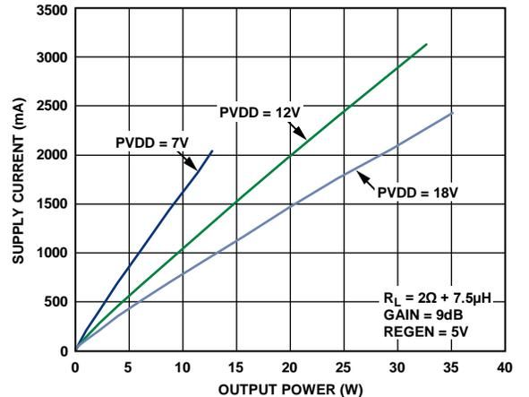
Figure 25. Supply Current vs. Output Power into 2Ω;
