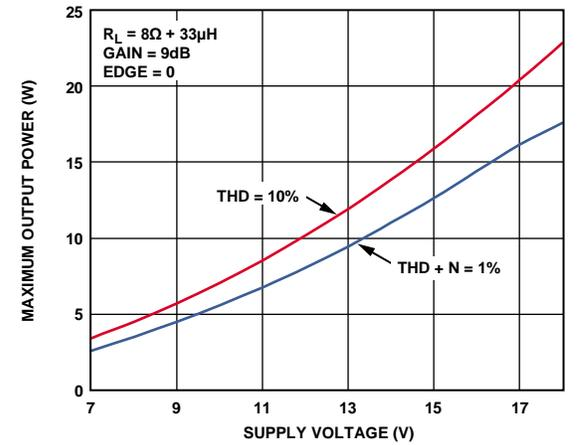
Figure 20. Maximum Output Power vs. Supply Voltage;
