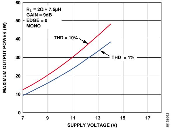
Figure 22. Maximum Output Power vs. Supply Voltage;
