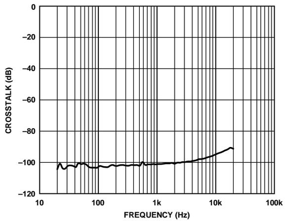
Figure 34. Crosstalk vs. Frequency,
