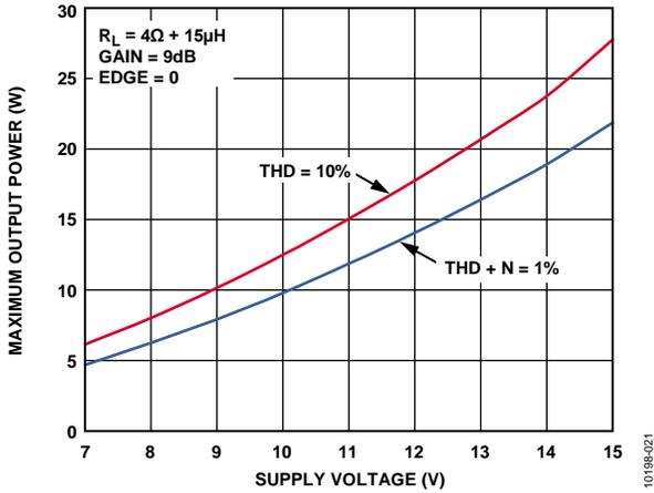
Figure 21. Maximum Output Power vs. Supply Voltage;
