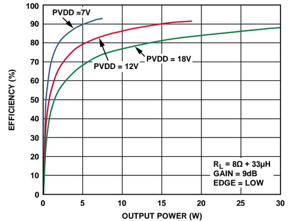
Figure 26. Efficiency vs. Output Power into 8Ω;
