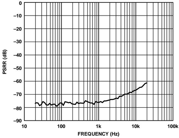
Figure 33. PSRR vs. Frequency,  $V_{RIPPLE} = 100\text{ mV rms}$
