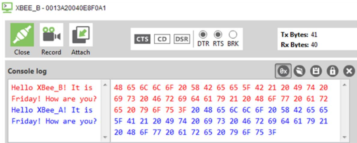
7. To disconnect, click the **Close serial connection** button
