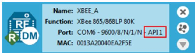
6. Select **XBEE\_A** and click the **Discover radio nodes in the same network** button
