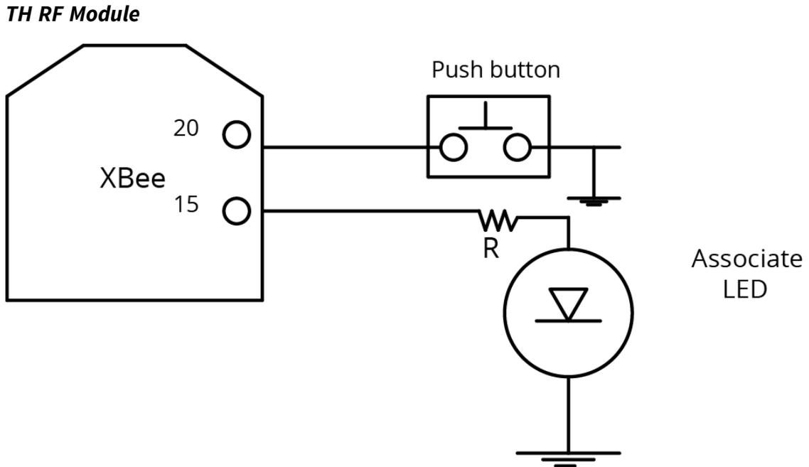
A pushbutton and an LED can be connected to the XBee 868LP RF Module pins 33 and 28 (SMT), or pins 20 and 15 (TH) respectively to support the commissioning pushbutton and associate LED functionalities.
