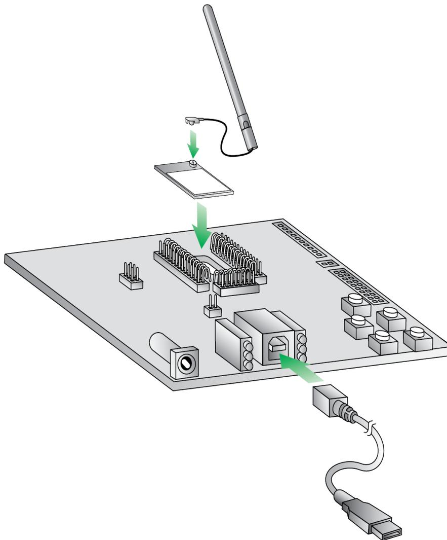
1. Attach the XBee 868LP RF Modules to the development boards.
