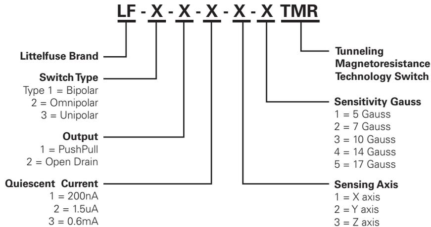
Example: LF21215TMR is an Omnipolar, PushPull, 1.5uA, X axis, 17 Gauss
