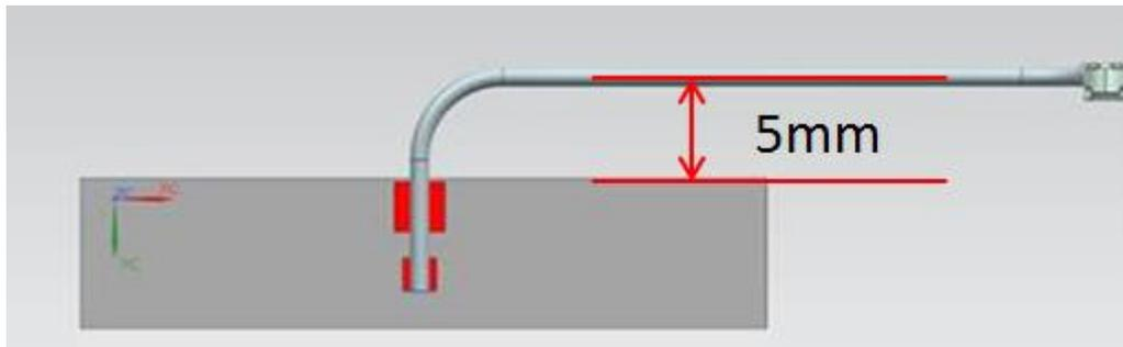
FIGURE 7.2 CABLE BENDING
