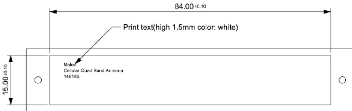
FIGURE 1. DIMENSION OF CELLULAR QUAD BAND FLEX ANTENNA
