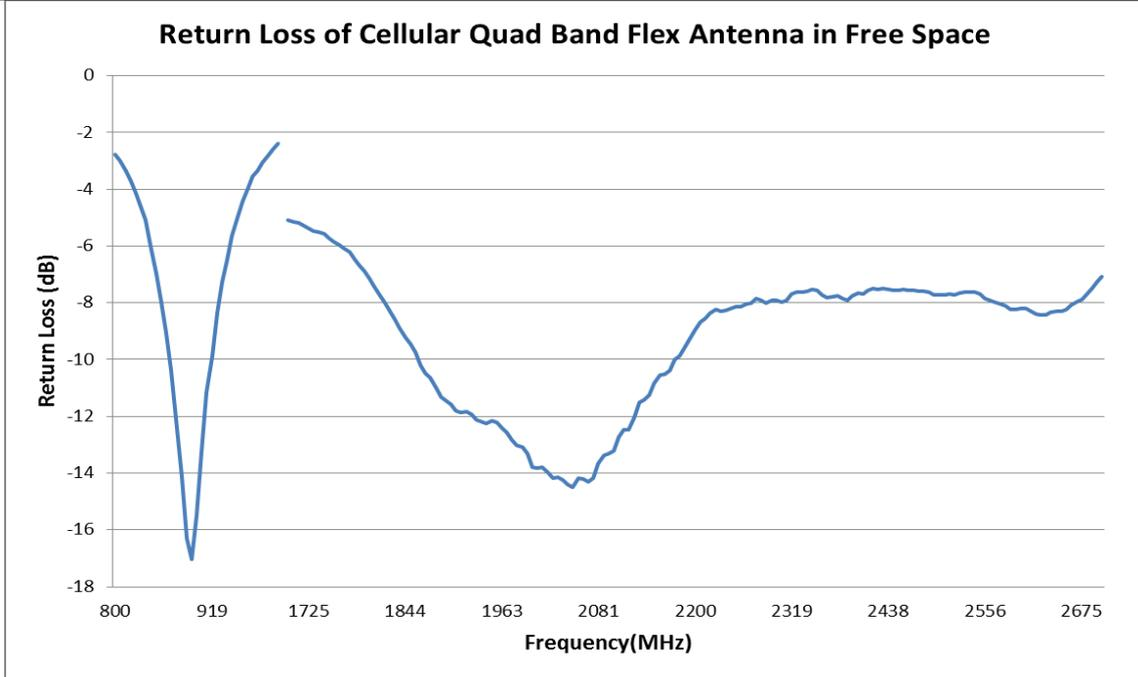
**FIGURE 2.2 RETURN LOSS OF ANTENNA IN FREE SPACE**
