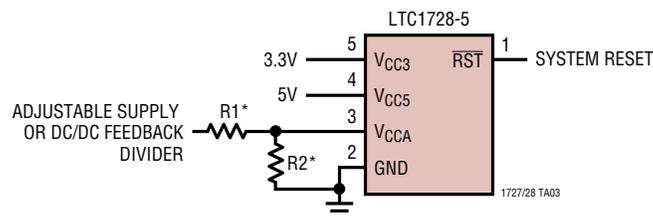
\*TO PRESERVE THRESHOLD ACCURACY, SET PARALLEL COMBINATION OF R1 AND R2  $\leq 66.5\text{k}$
