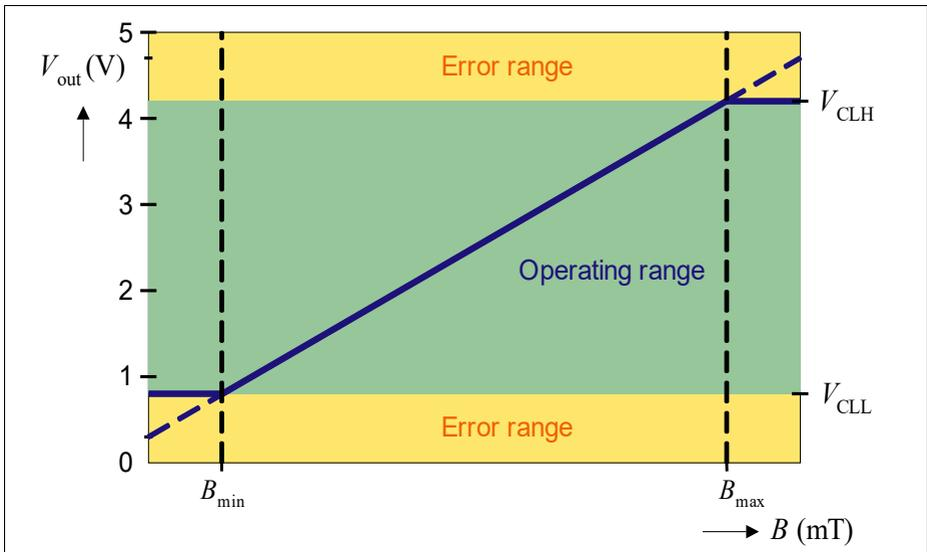
**Figure 8 Clamping Example**
