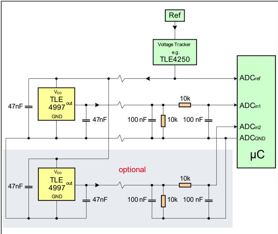
Figure 10 Application Circuit
