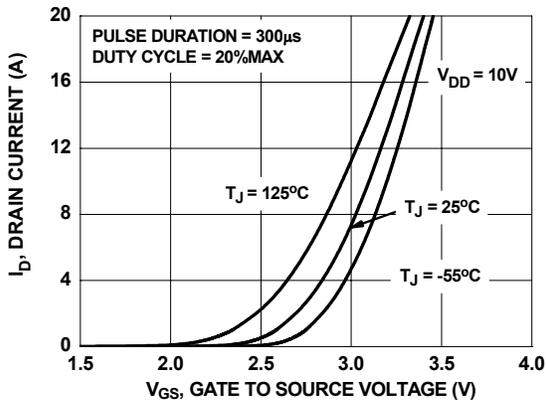
Figure 5. Transfer Characteristics
