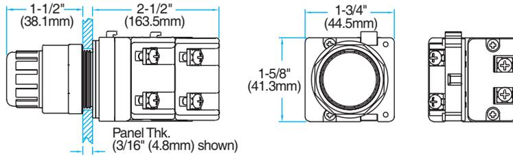
**FULL VOLTAGE & RESISTOR PUSH-TO-TEST OPERATORS (SHOWN WITH IPBCM)**
