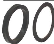
Our panel gaskets are constructed of Neoprene for long life and low compression set and provide a watertight seal. Panel gaskets are supplied to accommodate different panel thickness. In order to meet Type 4/4X requirements, at least one 1/16" (1.6mm) gasket must be used. NOTE: All c3controls 30mm operators are provided with gaskets.
