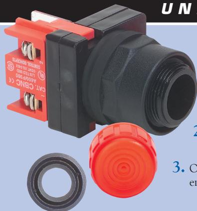
1. Our revolutionary U-Cup seal is infused with a Teflon coating to eliminate cracking when exposed to harsh conditions such as heat, dryness and sunlight. The U-Cup seal rides easily along the stroker and keeps water, oils, dust and other corrosive particles in the air away from the contact blocks. This U-cup seal also acts like a squeegee and forms a permanent watertight seal that meets Type 4/4X standards.
