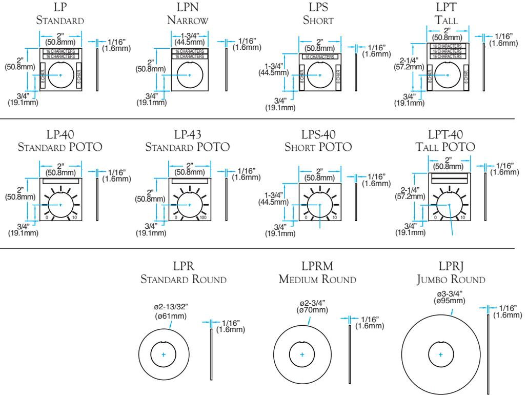
Note: Legend plates feature a tab for optional break-away positioning and can be used in conjunction with the Thrust & Trim Washer accessory.
