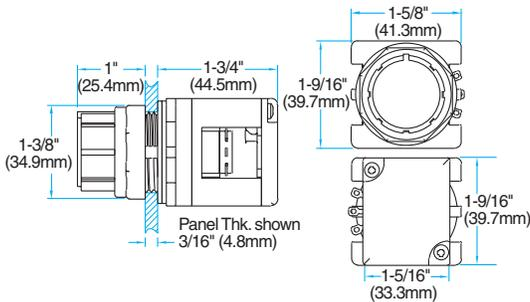
POTENTIOMETER OPERATOR (SHOWN WITH TERMINAL BLOCK)
