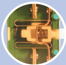
**NOTE:** Gold plated contacts are available on standard blocks for dry circuit applications. The cover will be gold (amber) in place of clear.
