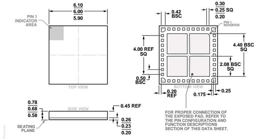
Figure 35. 40-Terminal Land Grid Array [LGA]
