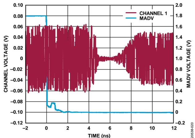
Figure 18. 25 GHz RF Frequency Band Switching with MADV
