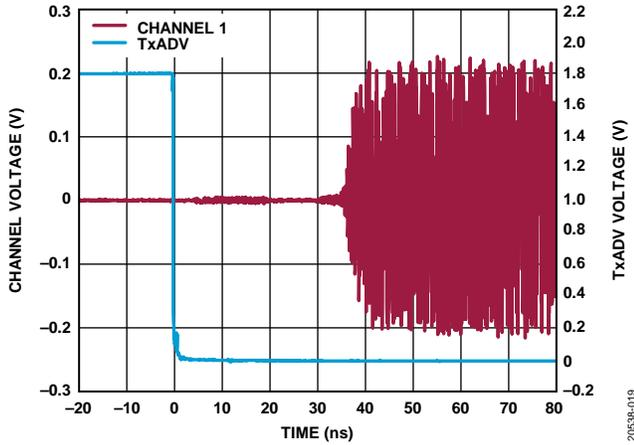
Figure 19. RF Output Sleep to Active Switching Time
