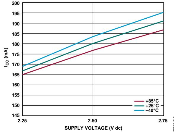
Figure 10.  $I_{cc}$  vs. Supply Voltage and Temperature
