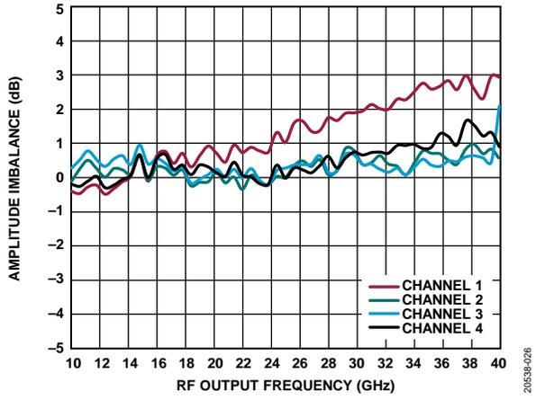
Figure 25. Amplitude Imbalance vs. RF Output Frequency
