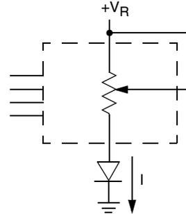
Two terminal Variable Resistor;
