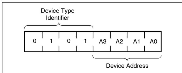
The next four bits of the slave address are the device address. The physical device address is defined by the state of the  $A_0 - A_3$  inputs. The X9418 compares the serial data stream with the address input state; a successful compare of all four address bits is required for the X9418 to respond with an acknowledge. The  $A_0 - A_3$  inputs can be actively driven by CMOS input signals or tied to  $V_{CC}$  or  $V_{SS}$ .
