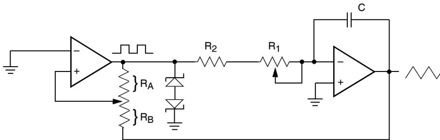
$$\text{frequency} \propto R_1, R_2, C$$
