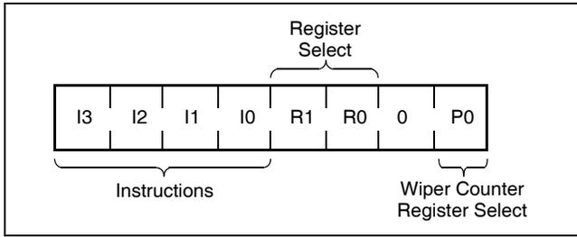
The four high order bits define the instruction. The next two bits (R1 and R0) select one of the four registers that is to be acted upon when a register oriented instruction is issued. The last bits (P0) select which one of the two potentiometers is to be affected by the instruction. Bit 1 is defined to be 0.
