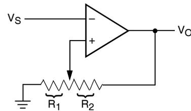
$$V_{UL} = \{R_1/(R_1 + R_2)\} V_O(max)$$
