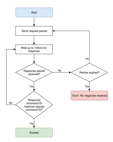
The values used for timeout or number of retries should be tuned to the specific application.
