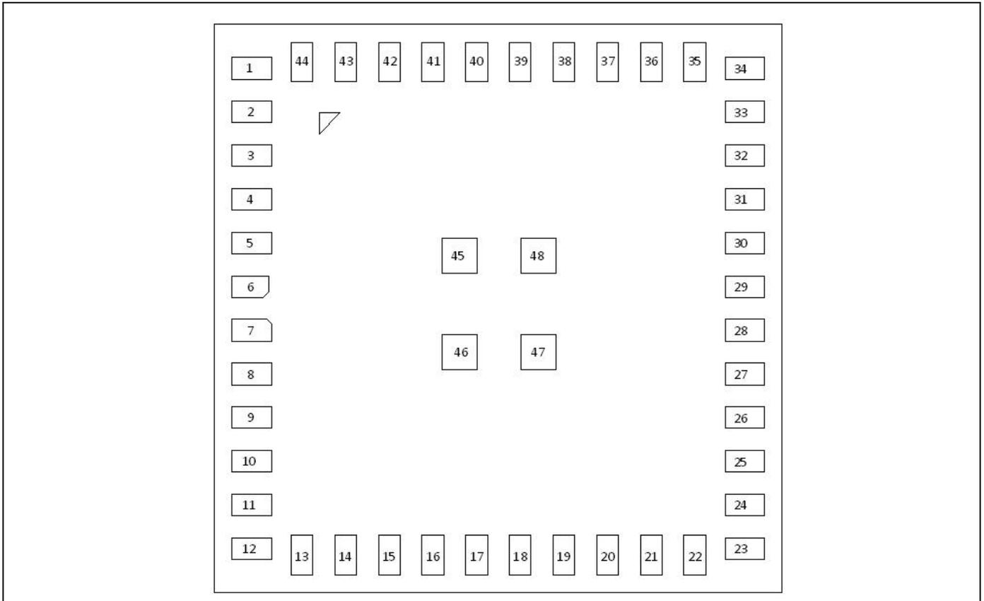
The signal name, type, and description of each pin in the CYW20737S is listed in [Table 3 on page 6](#). The symbols shown under I/O Type indicate pin directions (I/O = bidirectional, I = input, O = output) and the internal pull-up/pull-down characteristics (PU = weak internal pull-up resistor and PD = weak internal pull-down resistor), if any.
