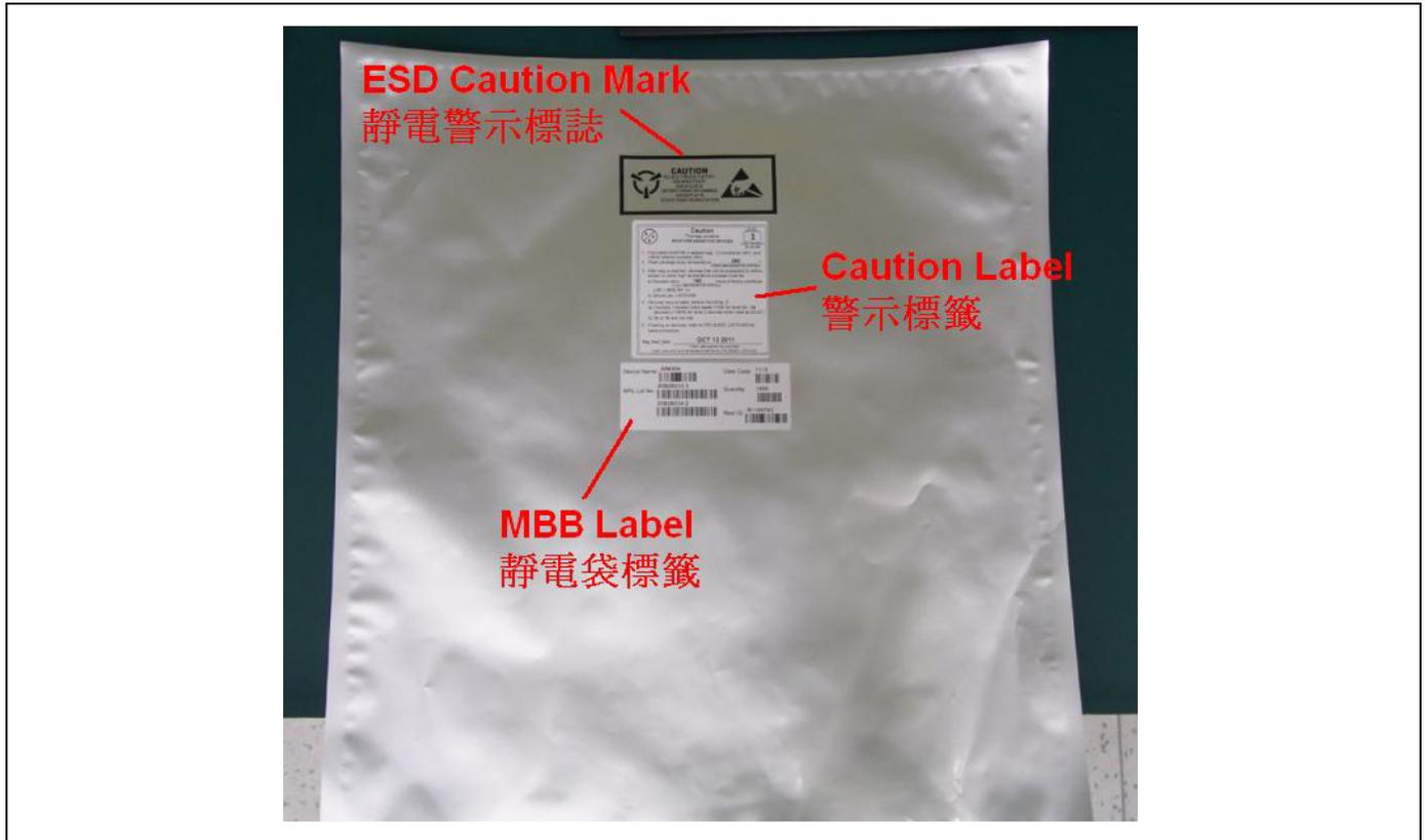
The moisture sensitivity label on the CYW20737S shipping bag is shown in [Figure 12](#) on page 19.
