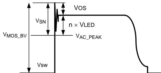
**Figure 24. Snubber Waveform**
