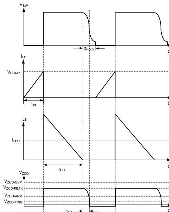
**Figure 15. Primary and Secondary Side Current Waveforms**
