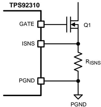
Figure 21.  $R_{ISNS}$  Resistor Interface
