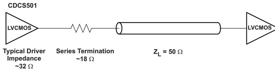
Figure 3. Test Load for 50-Ω Board Environment
