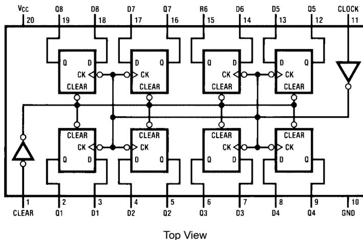
Figure 1. Pin Assignments for SOIC and TSSOP
