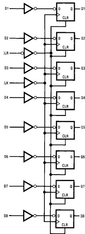
**Figure 2. Logic Diagram**
