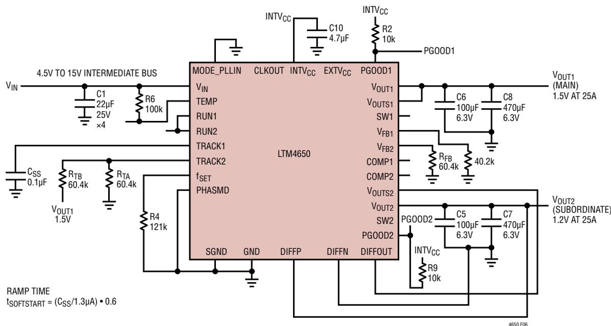
Figure 6. Example of Output Tracking Application Circuit
