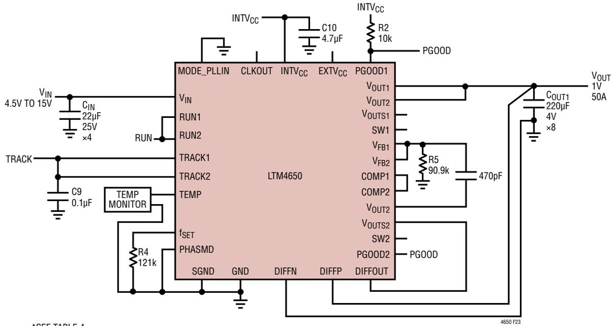
Figure 23. LTM4650 2-Phase, 1V at 50A Design
