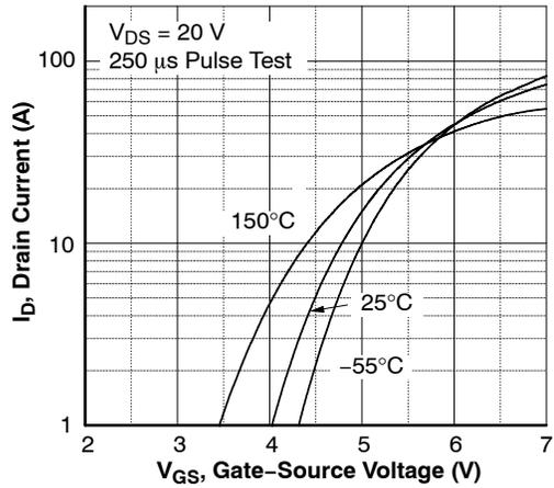
Figure 2. Transfer Characteristics
