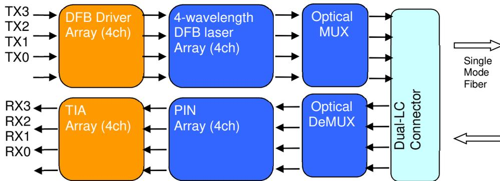
Figure 1: 40Gb/s QSFP LR4 Transceiver Block Diagram
