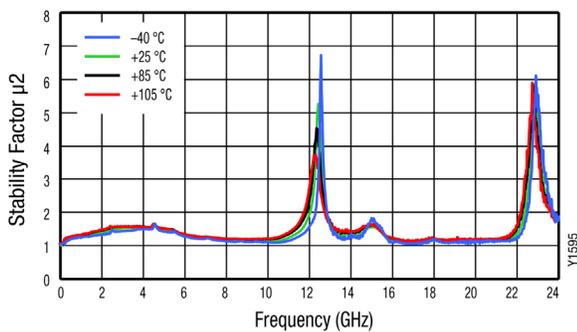
**Figure 13. Stability Factor ( $\mu_2$ ) vs Frequency over Temperature**
