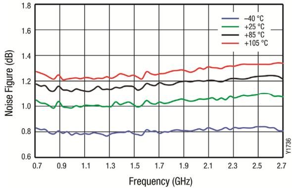
Figure 3. Evaluation Board NF vs Frequency over Temperature
