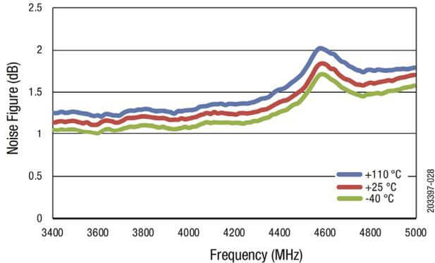
**Figure 28. Evaluation Board NF vs Frequency over Temperature**
