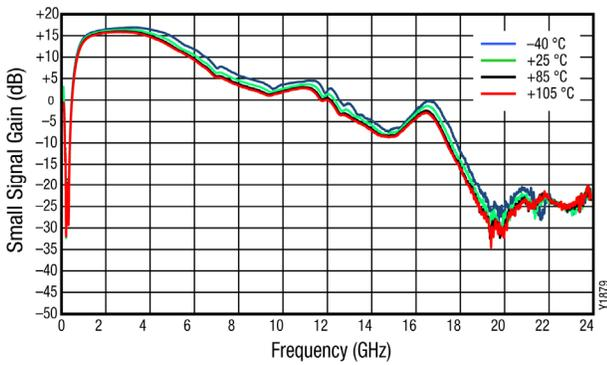
**Figure 19. Broadband Gain vs Frequency over Temperature**
