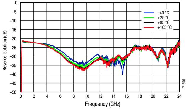
**Figure 9. Broadband Reverse Isolation vs Frequency over Temperature**
