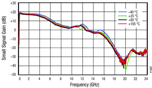
Figure 5. Broadband Gain vs Frequency over Temperature
