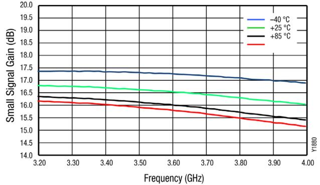
**Figure 20. Narrow Band Gain vs Frequency over Temperature**
