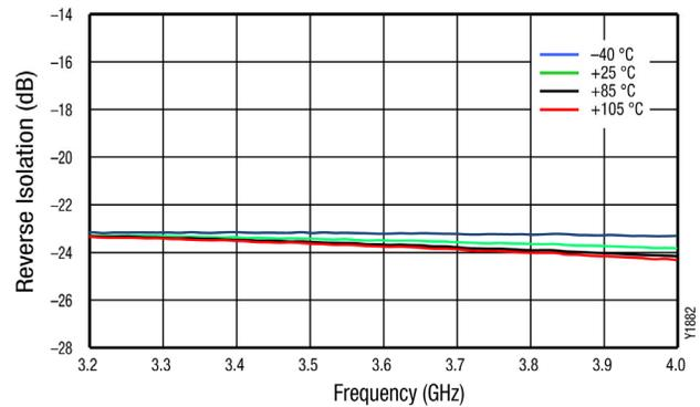
**Figure 22. Narrowband Reverse Isolation vs Frequency over Temperature**
