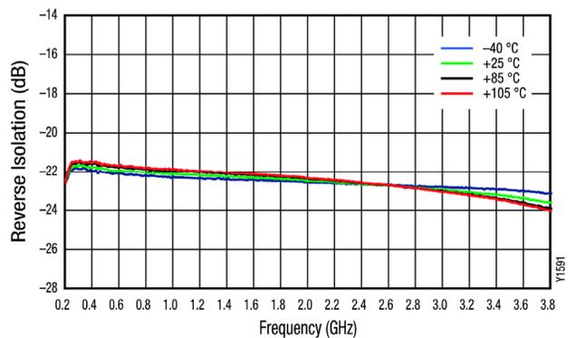
Figure 8. Narrowband Reverse Isolation vs Frequency over Temperature
