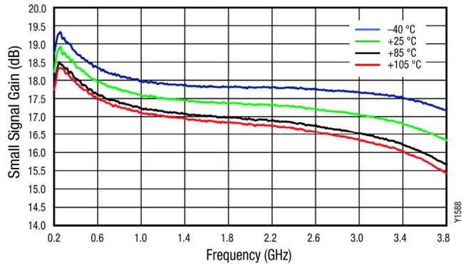
Figure 4. Narrow Band Gain vs Frequency over Temperature
