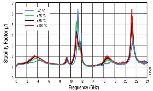
**Figure 12. Stability Factor ( $\mu_1$ ) vs Frequency over Temperature**
