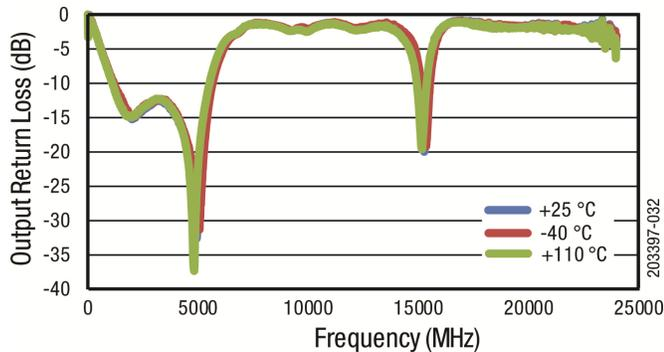
**Figure 32. Output Return Loss vs Frequency over Temperature**
