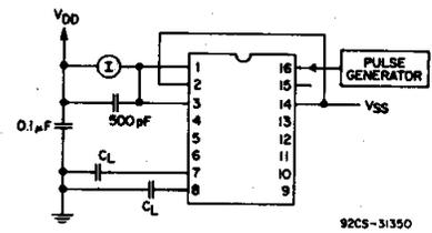
Fig. 15 - Dynamic power dissipation test circuit.
