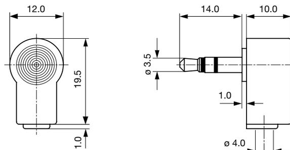
Cable diameter max. 4.0 mm
