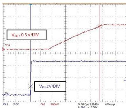
$V_{IN} = 2 \text{ V}$ ;  $V_O = 1 \text{ V}$ ;  $I_{OUT} = 1 \text{ mA}$
