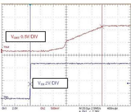
$V_{IN} = 2 \text{ V}$ ;  $V_O = 1 \text{ V}$ ;  $I_{OUT} = 150 \text{ mA}$
