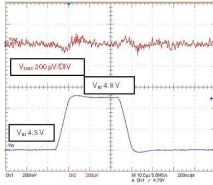
$V_{IN}$  = from 4.3 to 4.8 V;  $I_{OUT} = 1 \text{ mA}$ ;  $t_{rise} = t_{fall} = 5 \mu s$
