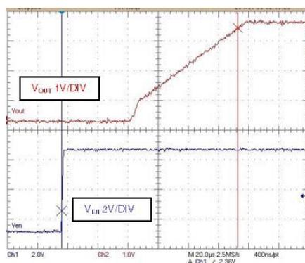
$V_{IN} = 4.3 \text{ V}$ ;  $V_O = 3.3 \text{ V}$ ;  $I_{OUT} = 1 \text{ mA}$
