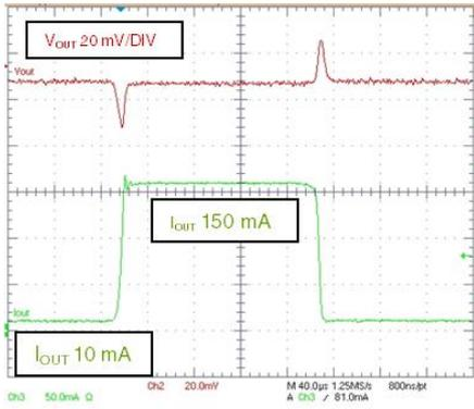
$I_{OUT}$  = from 10 to 150 mA;  $t_{rise} = t_{fall} = 5 \mu s$
