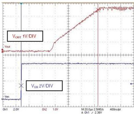
$V_{IN} = 4.3\text{ V}$ ;  $V_O = 3.3\text{ V}$ ;  $I_{OUT} = 150\text{ mA}$
