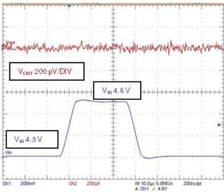
$V_{IN}$  = from 4.3 to 4.8 V;  $I_{OUT} = 150 \text{ mA}$ ;  $t_{rise} = t_{fall} = 5 \mu s$
