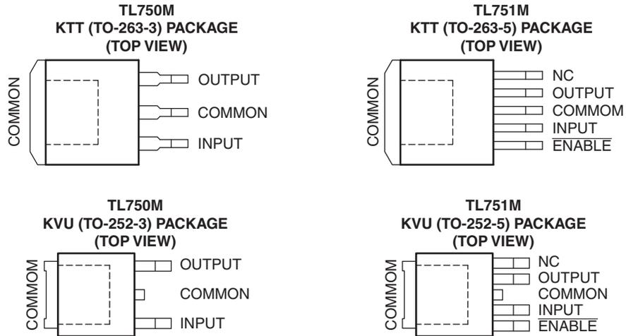
NOTE: The COMMON terminal is in electrical contact with the mounting base.
