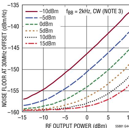
**Output Noise Floor vs RF Output Power and Differential LO Input Power**
