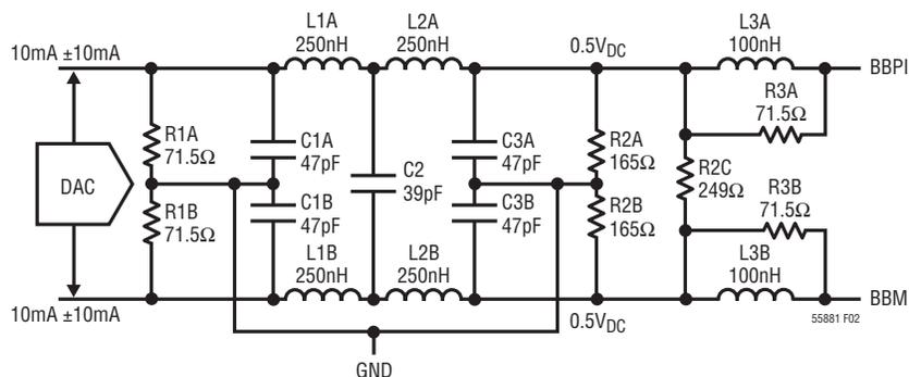
**Figure 2: Baseband Interface with 5th-Order Filter and 0.5V<sub>CM</sub> DAC (Only I Channel is Shown)**
