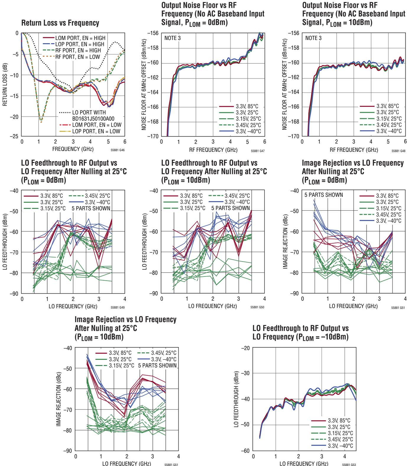
**TYPICAL PERFORMANCE CHARACTERISTICS**  $V_{CC} = 3.3V$ ,  $EN = 3.3V$ ,  $T_A = 25^\circ C$ , LOP input AC-terminated with  $50\Omega$  to ground, BBPI, BBMI, BBPQ, BBMQ inputs  $0.5V_{DC}$ , and  $1V_{P-P(DIFF)}$ , baseband input frequencies = 4.5MHz and 5.5MHz for OIP3 and OIP2, or else baseband input frequency = 100kHz, I and Q  $90^\circ$  shifted, lower sideband selection, LINOPT pin floating, unless otherwise noted. Test circuit is shown in Figure 8.
