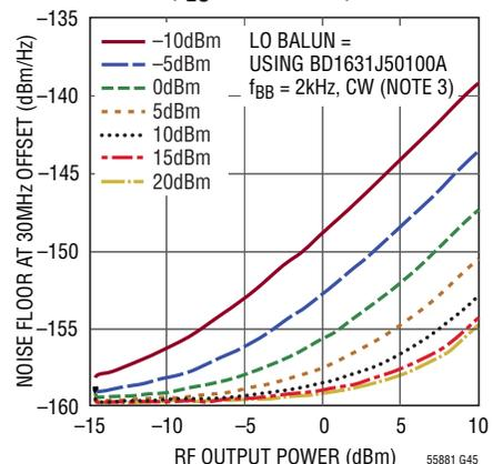
**TYPICAL PERFORMANCE CHARACTERISTICS**  $V_{CC} = 3.3V$ ,  $V_{EN} = 3.3V$ ,  $T_A = 25^\circ C$ , LOP input AC-terminated with  $50\Omega$  to ground, BBPI, BBMI, BBPQ, BBMQ inputs  $0.5V_{DC}$ , and  $1V_{P-P(DIFF)}$ , baseband input frequencies = 4.5MHz and 5.5MHz for OIP3 and OIP2, or else baseband input frequency = 100kHz, I and Q  $90^\circ$  shifted, lower sideband selection, LINOPT pin floating, unless otherwise noted. Test circuit is shown in Figure 8.
