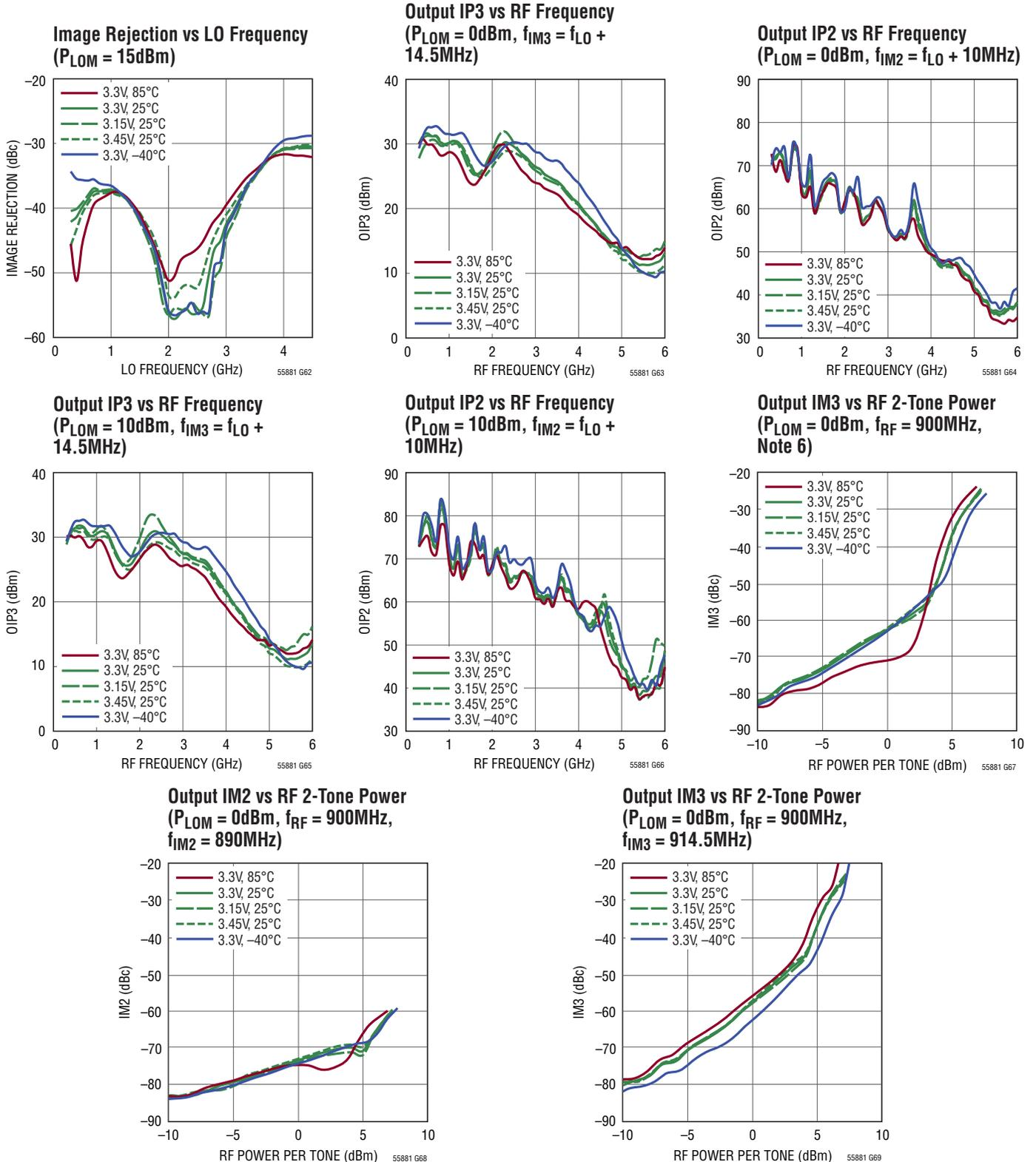
**TYPICAL PERFORMANCE CHARACTERISTICS**  $V_{CC} = 3.3V$ ,  $EN = 3.3V$ ,  $T_A = 25^\circ C$ , LOP input AC-terminated with  $50\Omega$  to ground, BBPI, BBMI, BBPQ, BBMQ inputs  $0.5V_{DC}$ , and  $1V_{P-P(DIFF)}$ , baseband input frequencies = 4.5MHz and 5.5MHz for OIP3 and OIP2, or else baseband input frequency = 100kHz, I and Q  $90^\circ$  shifted, lower sideband selection, LINOPT pin floating, unless otherwise noted. Test circuit is shown in Figure 8.
