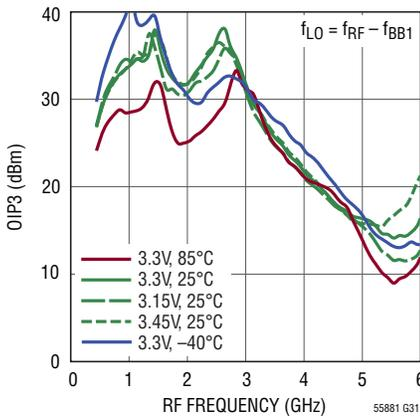
**Output IP3 vs RF Frequency for Low Side LO Injection**
