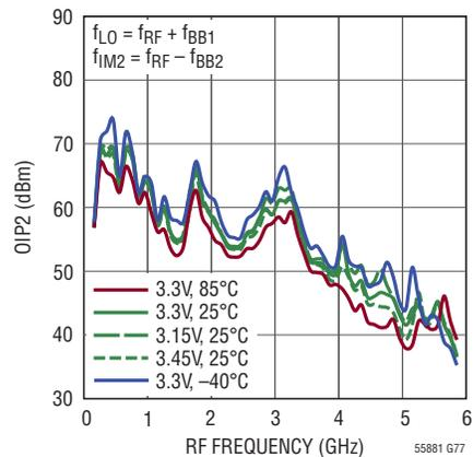
**TYPICAL PERFORMANCE CHARACTERISTICS**  $V_{CC} = 3.3V$ ,  $EN = 3.3V$ ,  $T_A = 25^\circ C$ , LOP input AC-terminated with  $50\Omega$  to ground, BBPI, BBMI, BBPQ, BBMQ inputs  $0.5V_{DC}$ , and  $1V_{P-P(DIFF)}$ , baseband input frequencies = 4.5MHz and 5.5MHz for OIP3 and OIP2, or else baseband input frequency = 100kHz, I and Q  $90^\circ$  shifted, lower sideband selection, LINOPT pin floating, unless otherwise noted. Test circuit is shown in Figure 8.
