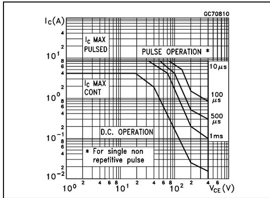
Figure 3. Derating curve
