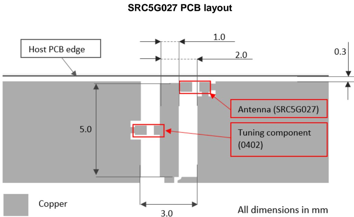
Below shows the PCB layout without solder mask for illustration purposes only.
