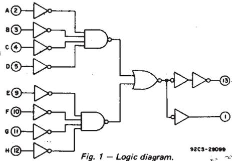
Fig. 1 - Logic diagram.
