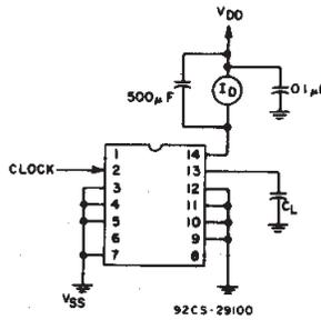
Fig. 14 – Dynamic power dissipation test circuit.
