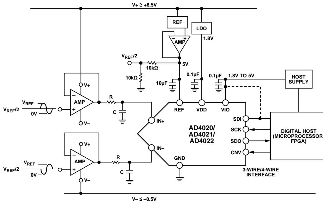
Figure 40. Typical Application Diagram with Multiple Supplies
