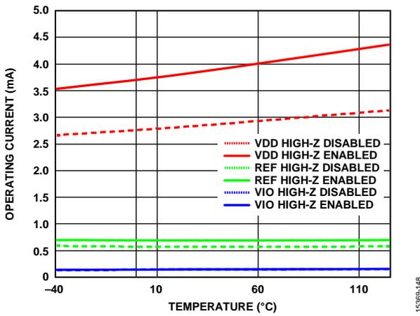
Figure 30. Operating Current vs. Temperature, AD4021, 1 MSPS
