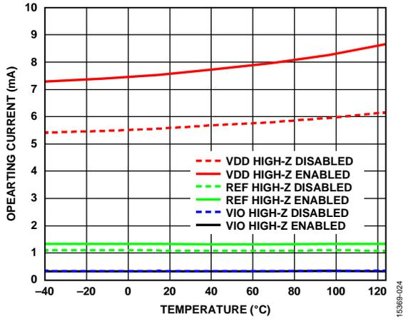
Figure 29. Operating Current vs. Temperature, AD4020, 1.8 MSPS
