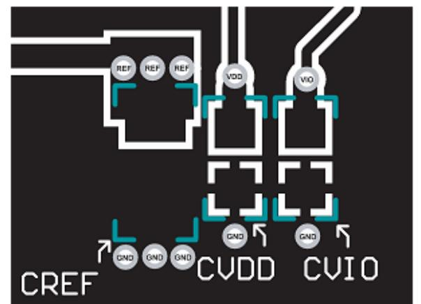
Figure 68. Example Layout of the AD4020 (Bottom Layer)
