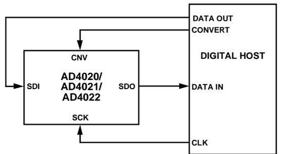
Figure 59. CS Mode, 4-Wire Turbo Mode Connection Diagram
