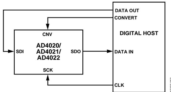
Figure 53. CS Mode, 3-Wire Turbo Mode Connection Diagram
