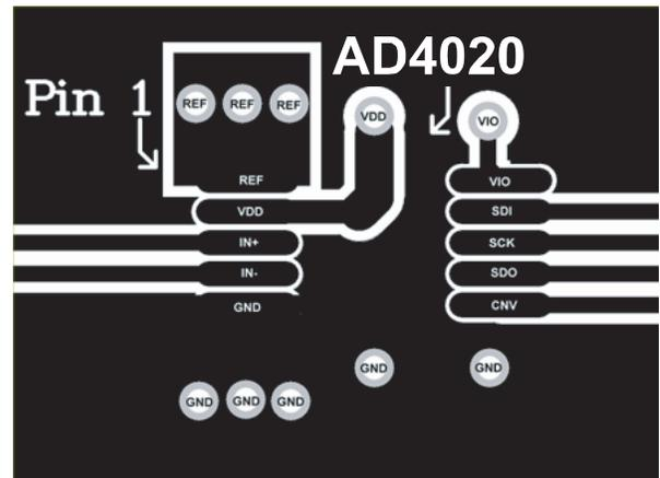
Figure 67. Example Layout of the AD4020 (Top Layer)
