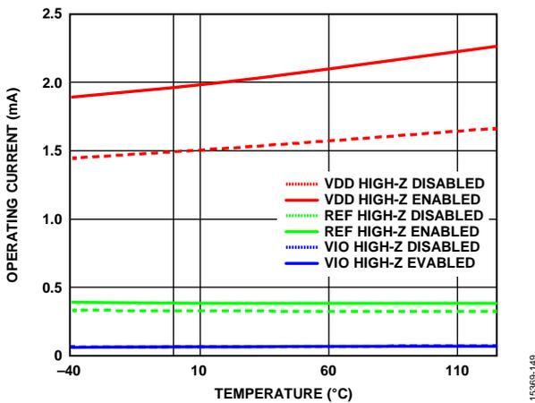
Figure 31. Operating Current vs. Temperature, AD4022, 500 kSPS
