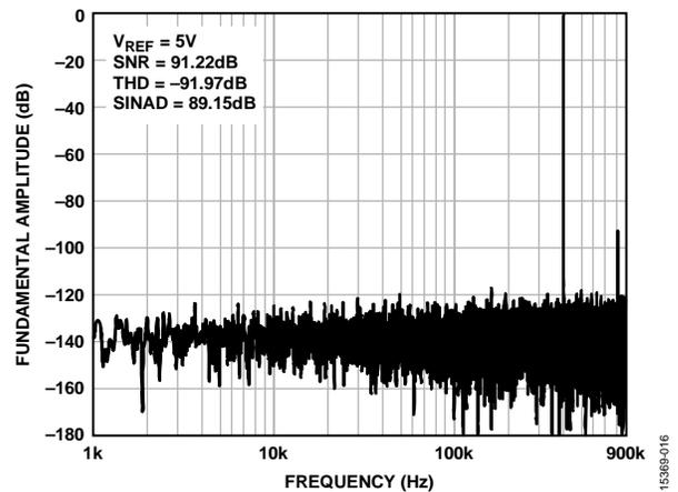
Figure 16. 400 kHz, -0.5 dBFS Input Tone FFT
