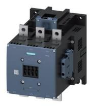
power contactor, AC-3 400 A, 200 kW / 400 V AC (50-60 Hz) / DC operation 200-277 V AC/DC auxiliary contacts 2 NO + 2 NC 3-pole, frame size S12 busbar connections drive: electronic with PLC interface 24 V DC screw terminal
