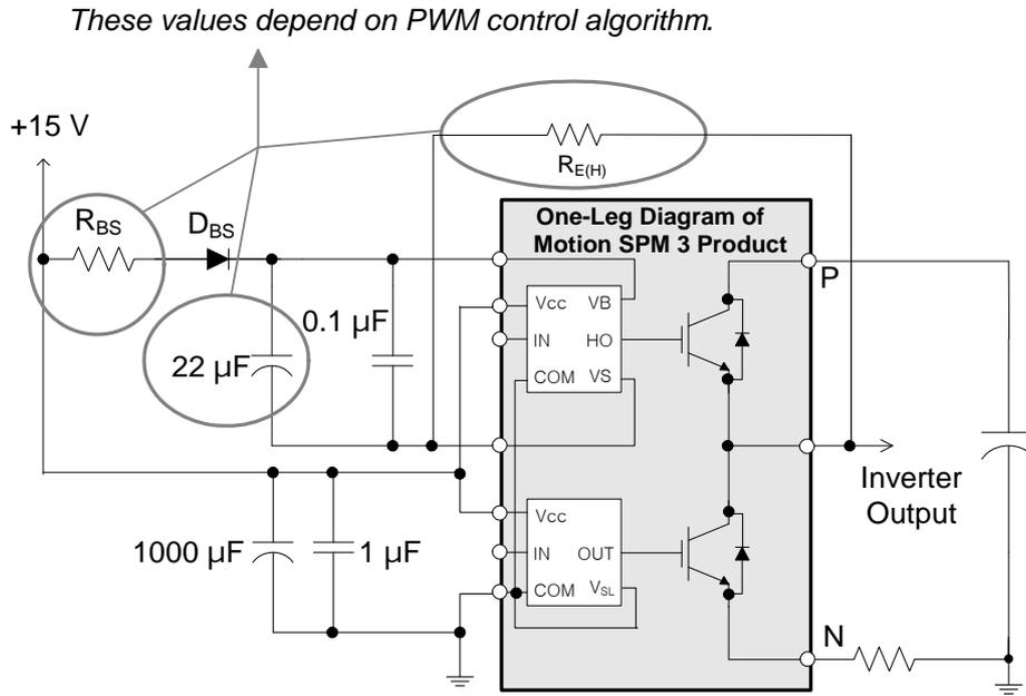
**Figure 10. Recommended Bootstrap Operation Circuit and Parameters**
