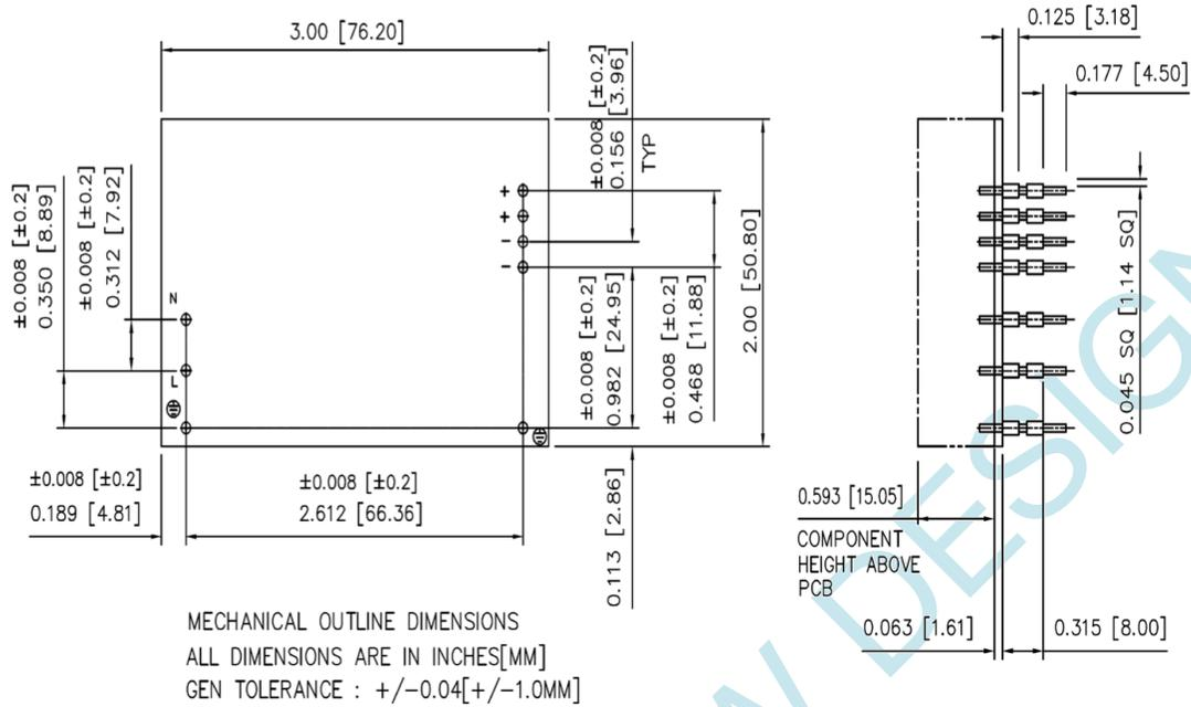
Figure 4. Mechanical Drawing – PCB Mount Option
