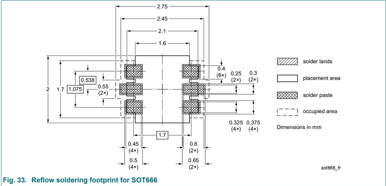
Fig. 33. Reflow soldering footprint for SOT666
