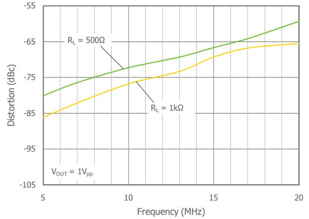
2nd Harmonic Distortion vs.  $V_{OUT}$  at  $V_S = 5\text{V}$
