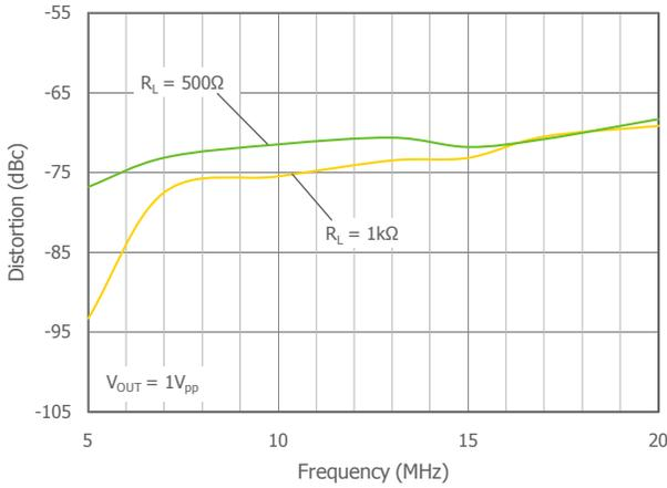
3rd Harmonic Distortion vs.  $R_L$  at  $V_S = 5\text{V}$
