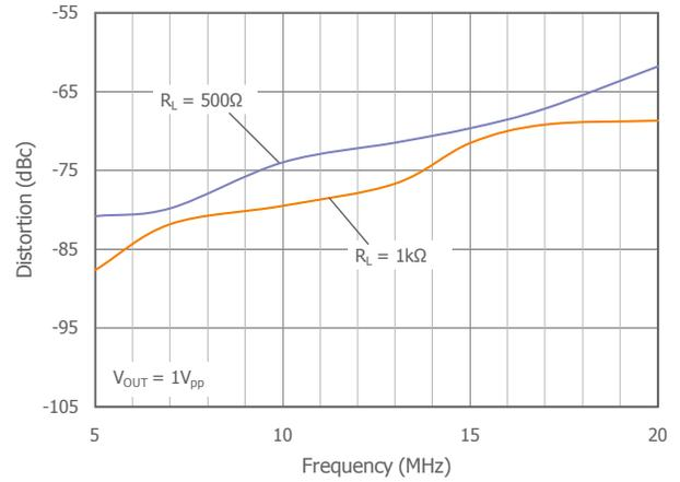
2nd Harmonic Distortion vs.  $V_{OUT}$
