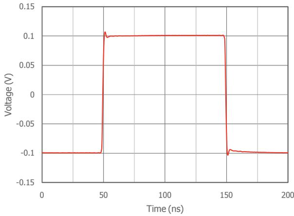
Small Signal Pulse Response at  $V_S = 5\text{V}$
