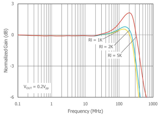
Frequency Response vs.  $V_{OUT}$
