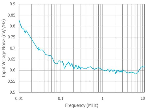
Input Voltage Noise at  $V_S = 5\text{V}$  (>10kHz)
