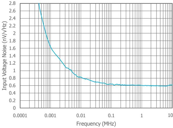
Input Voltage Noise at  $V_S = 5\text{V}$
