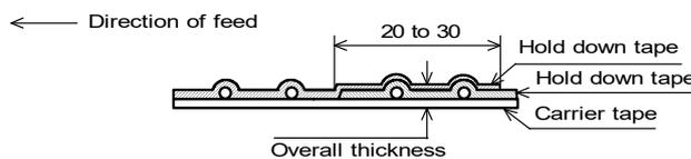
· Hold down tape shall be spliced with overlapping.
