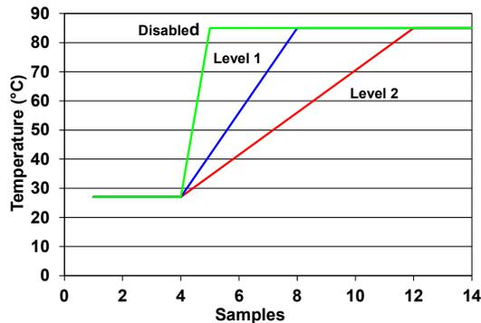
**Figure 7-4. Temperature Filter Impulse Response**
