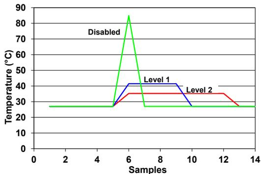
The filter consists of a running average on the external diode channel. The Level 1 filter is a running average of 4x while the Level 2 filter is a running average of 8x. For the first measurement immediately after power-up, the filter will be filled with the results of the first measurement. After this, the filter is operated normally. Any temperature comparisons are done with the filtered results that are stored in the user register.
