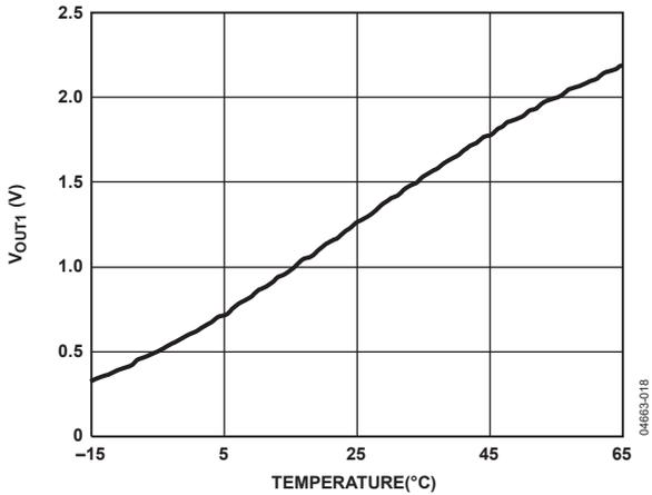
Figure 18. V<sub>OUT1</sub> vs. Temperature
