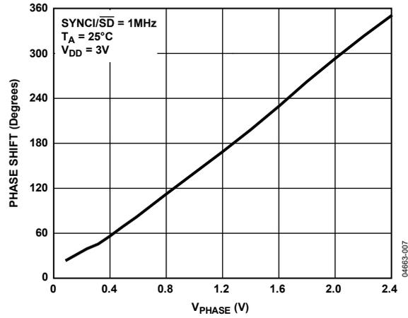
Figure 7. Clock Phase Shift vs. Phase Voltage
