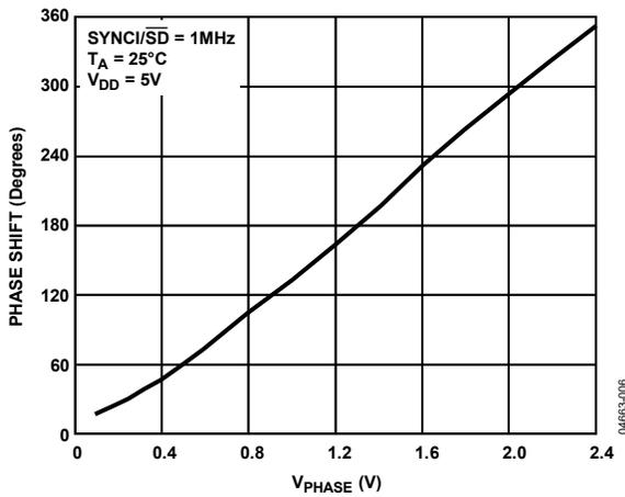
Figure 6. Clock Phase Shift vs. Phase Voltage
