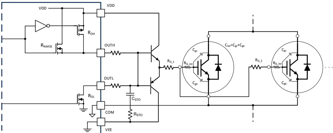
Figure 54. Current Buffer for Increased Drive Strength
