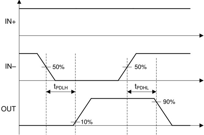
**Figure 26. Inverting Logic Propagation Delay Measurement**
