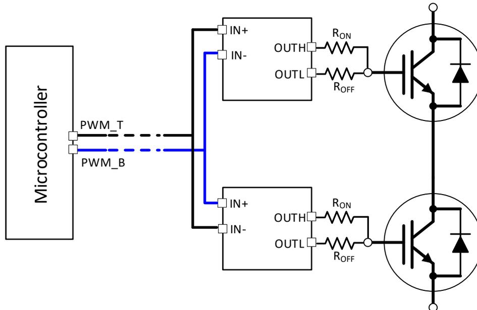
Figure 45. PWM Interlock for a Half Bridge
