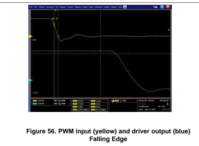
Figure 56. PWM input (yellow) and driver output (blue) Falling Edge
