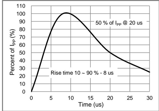
Fig.2 Pulse Waveform
