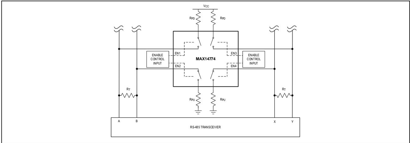
**RS-485 Termination Resistor Switch**
