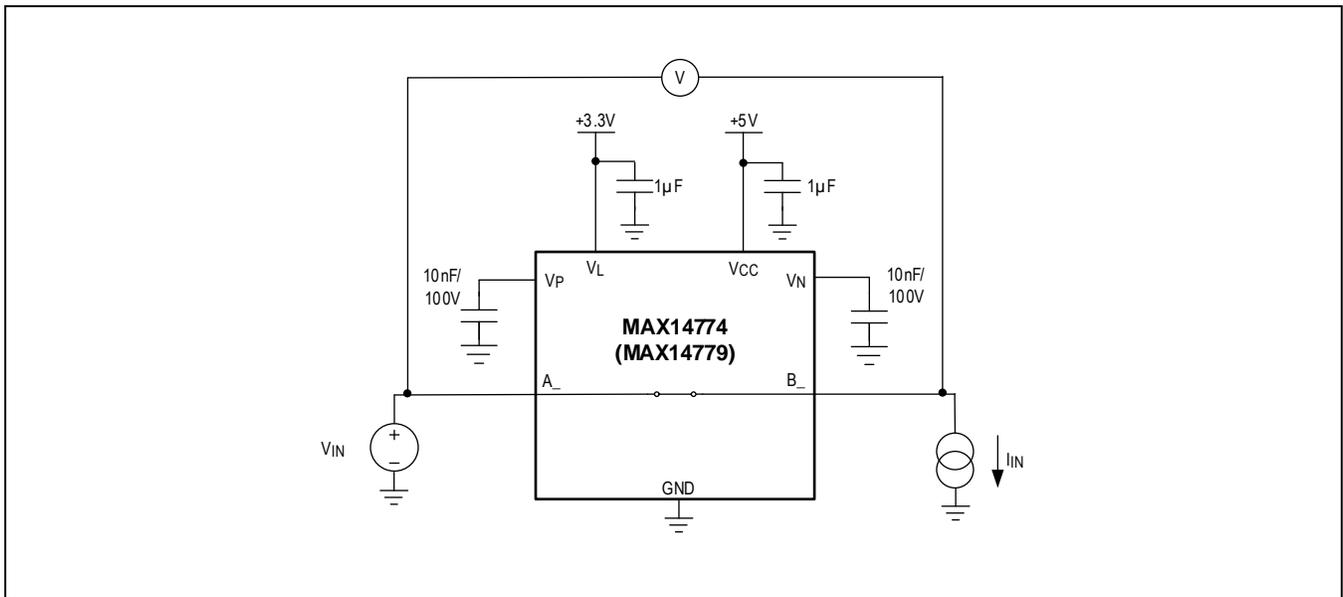
Figure 1. On-Resistance Measurement
