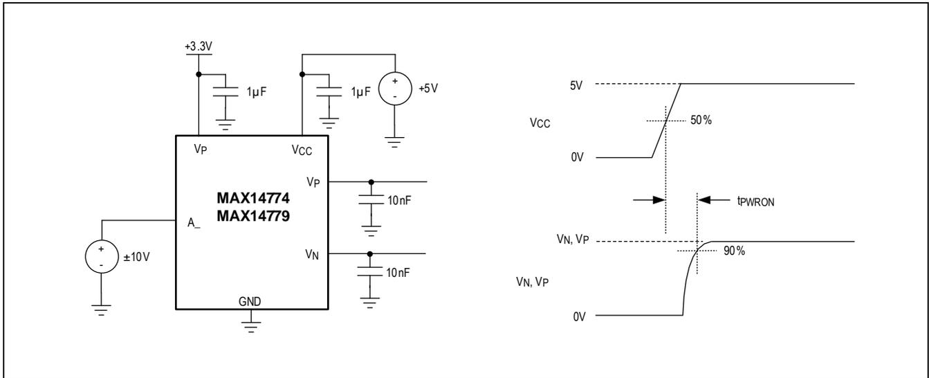
Figure 3. Power-Up Time Measurement
