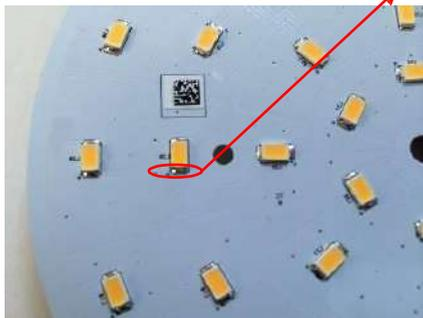
You can use the high-temperature thermal conductivity glue (Such as SatlonD-3/606...etc.) to fix the thermal couple to the solder joint then measure the temperature. Once you got the  $T_s$  temperature measurement data, you can calculate the junction temperature based on the measurement data of the  $T_s$ . The details of the calculation method are shown in the following page:
