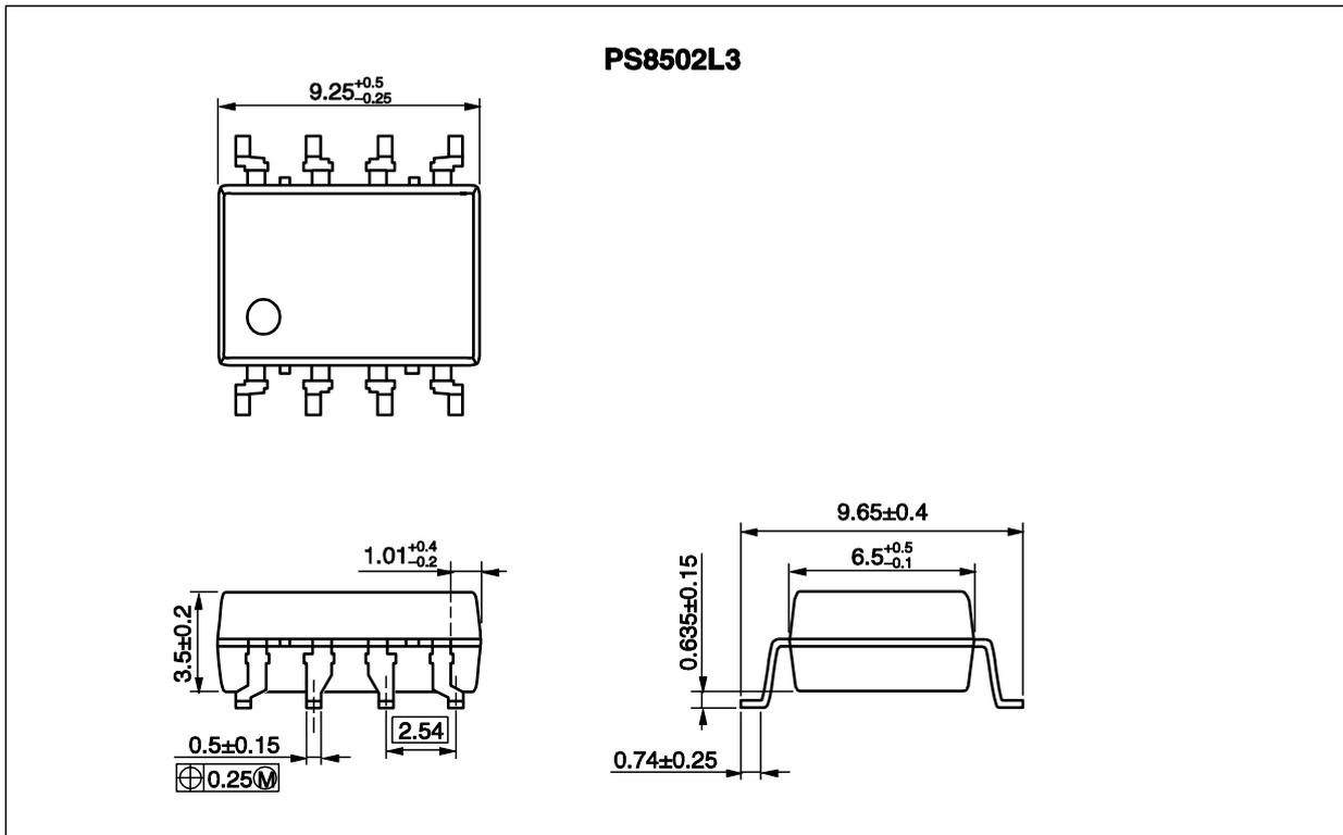
Lead Bending Type For Long Creepage Distance
