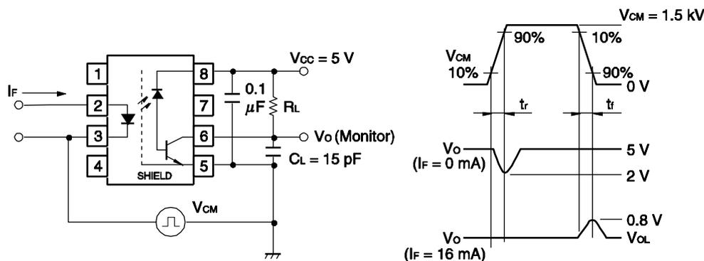
**Remark**  $C_L$  includes probe and stray wiring capacitance.
