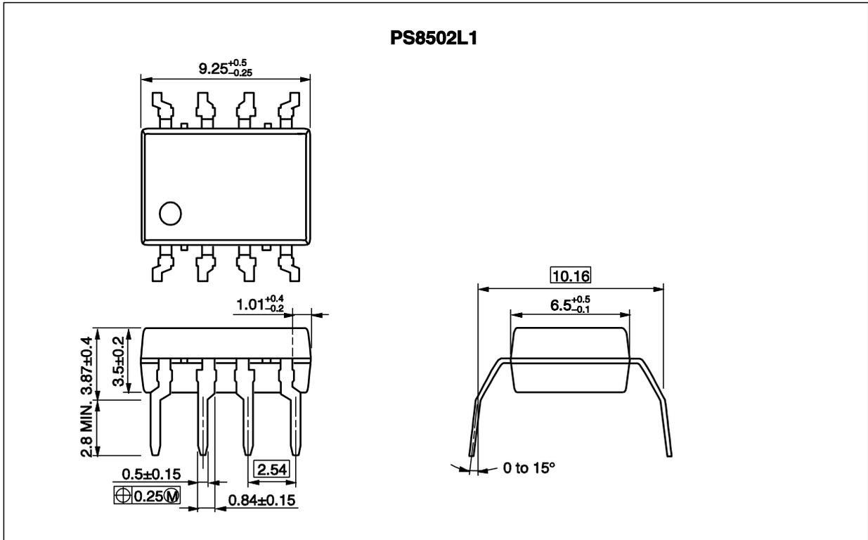
Lead Bending Type For Long Creepage Distance (Gull-wing) For Surface Mount
