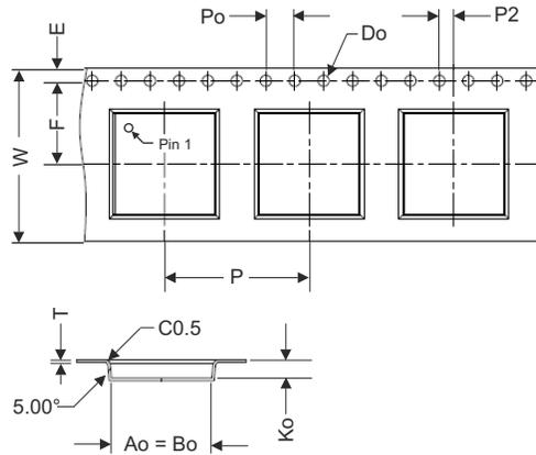
**Figure 12-2. Tape Specification**
