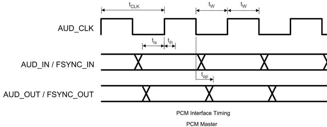
Figure 8-12. Bluetooth Codec-PCM (Audio) Master Timing Diagram
