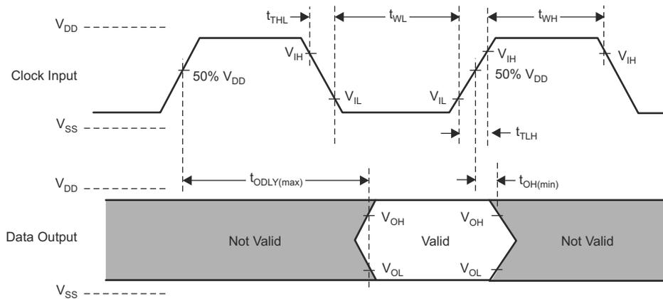
**Figure 8-9. SDIO HS Output Timing**
