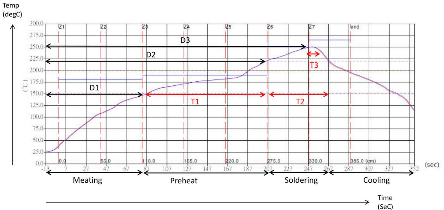
**Figure 10-7. Reflow Profile for the WiLink 8 Module**
