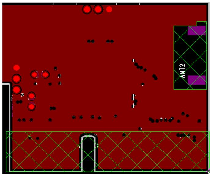
Figure 10-4. TI Module Layout: Layer 2 (Solid GND)
