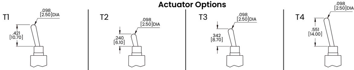
\* B4 bushing shown. Subtract 2.55mm from toggle length for B1 bushing.
